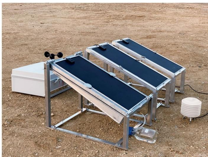
*In Thuwal, Saudi Arabia, a photovoltaic panel backed with a hydrogel that sucks water from the atmosphere stayed 10 °C cooler than those without and produced more electricity.*
