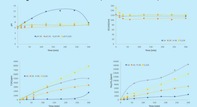
When evaluating different intensities, it is evident that intensity plays an important role on electrochemical CO<sub>2</sub> fixation, and pH values remain stable in all the experiments, although there is a pH increment in 1 A intensity, which suggest a slower fixation of CO<sub>2</sub>.
