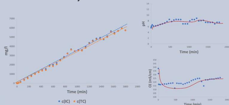
These results show that at 1 A intensity, CO<sub>2</sub> can be fixed along with the production of NaOH from the cathodic chamber, and pH (7-8) and electric conductivity values (CE, 120 mS/cm) remains stable along the experiment, suggesting the formation of carbonic acid and bicarbonate ions.
