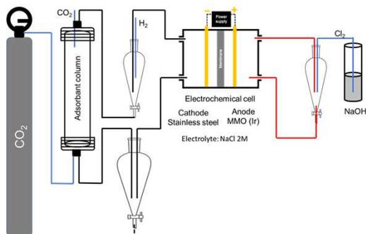
a 30 h duration experiment using a constant flow of CO<sub>2</sub> and 1 A intensity
