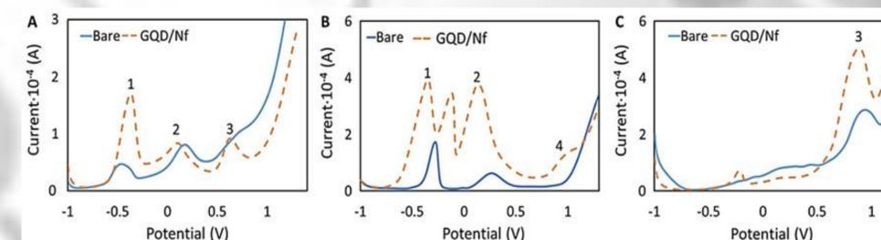
Voltammograms for Mincartil in 0.1 M KCl (A), Vitax in 0.05 M HNO<sub>3</sub> (B) and L-tyrosine BioTech (C) in 0.1 M KCl using the GQD/Nf electrodes. Peaks marked as 1, 2, 3 and 4 refer to the analytical signal of riboflavin, ascorbic acid, tyrosine, and pyridoxine, respectively.
