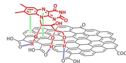
Interactions of GQD on the electrode surface and riboflavin as the target analyte.
